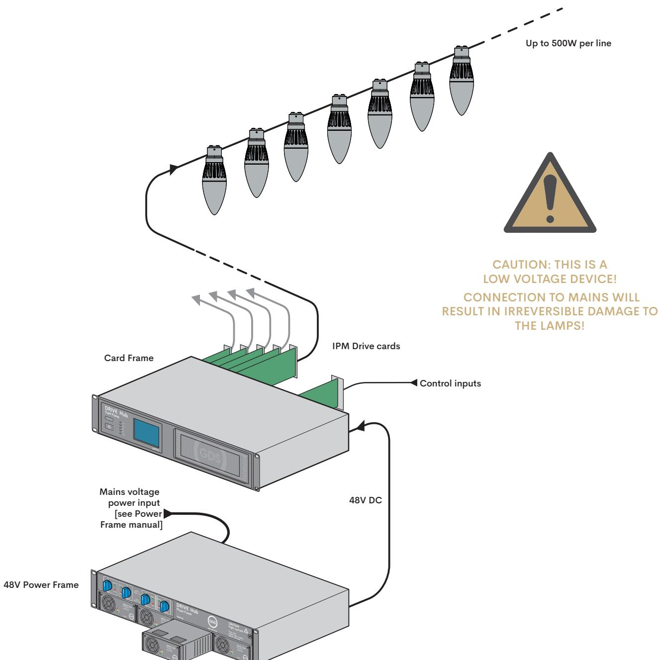
\*This example illustrates connection to the Card Frame and Power Frame via IPM Drive Cards. The GDS Lamp is also compatible with the Mini Pack and Micro Pack systems when used with IPM Drive Cards.
